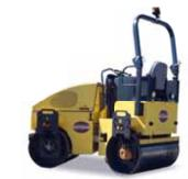
Rotating warning light and serial ROPS protection
