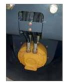
Lubrication point on each cylinder and Poclain drive motors
