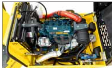
Turbo engine 44 hp to amplify extra power
