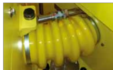
Double articulation with lubrication points 'Pac-Pivot' (patented)
