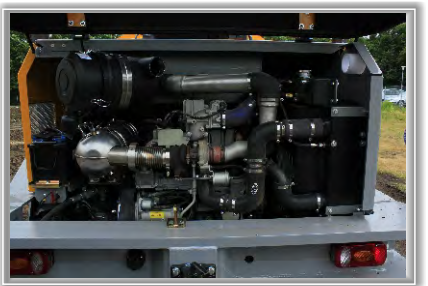
Readily accessible: Transversely installed engine
