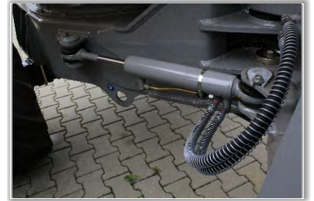
Robust: Steering cylinders attached with protection
