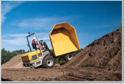
More flexibility: 90° rotating skip. Ideal in tight spaces.
