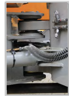
Robust: Steering cylinders attached with protection
